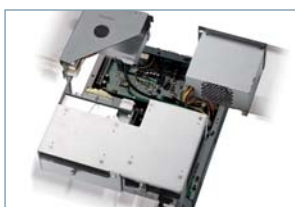
2. Modular design for easy maintenance
